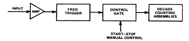
Figure 3-4. Electronic counter totalizing method, block diagram
