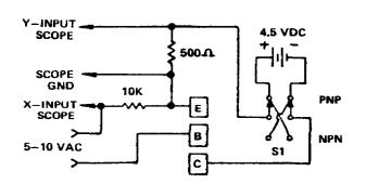
Figure 3-16. Transistor tester schematic
