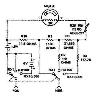
Figure 1-9. Circuit of a series ohmeter
