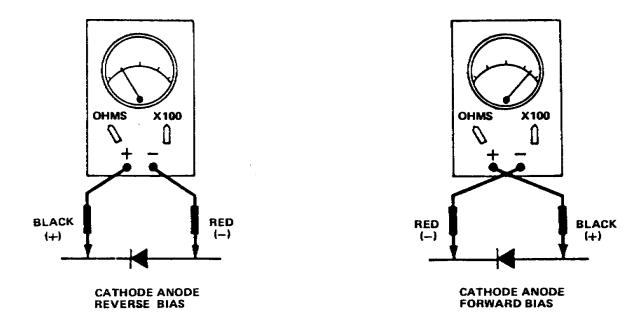
Figure 1-26. Forward-bias and reverse-bias diode
