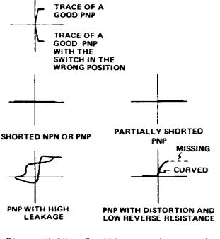
Figure 3-18. Oscilloscope traces of PNP transistors
