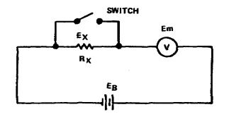
Figure 1-12. Determining value of unknown resistance of voltmeter
