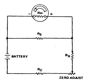
Figure 1-8. Typical ohmmeter circuit
