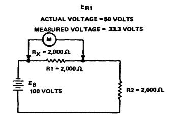
Figure 1-7. Error in voltmeter readings
