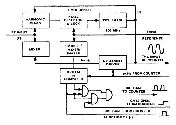
Figure 3-12. Electronic counter automatic method, block diagram
