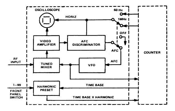
Figure 3-11. Electronic counter transfer oscillator method, block diagram
