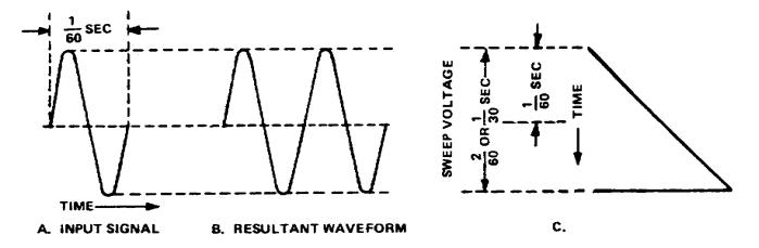
Figure 2-7. Sweep frequency lower than test signal frequency
