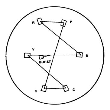
Figure 3-35. Typical vector display oscilloscope pattern
