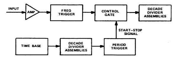
Figure 3-5. Electronic counter frequency measurement, block diagram
