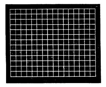
Figure 3-21. Grating test pattern
