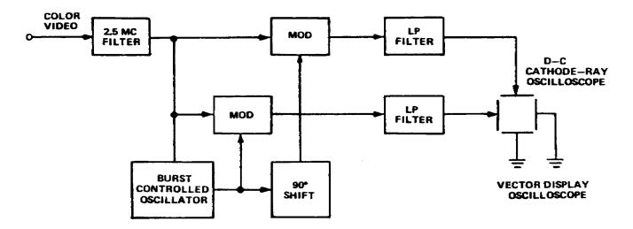
Figure 3-34. Block diagram of a typical vector display oscilloscope
