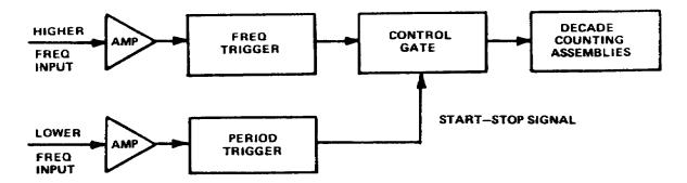
Figure 3-7. Electronic counter ratio measurement, block diagram
