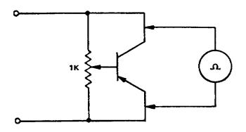
Figure 1-27. False ohmmeter reading
