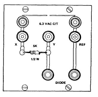
Figure 3-14. Locally manufactured diode tester
