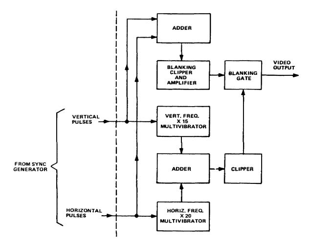
Figure 3-22. Grating generator, block diagram
