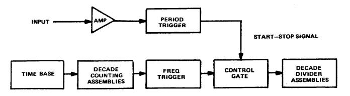
Figure 3-6. Electronic counter period measurement, block diagram
