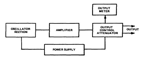
Figure 3-2. Block diagram of audio or video signal generator
