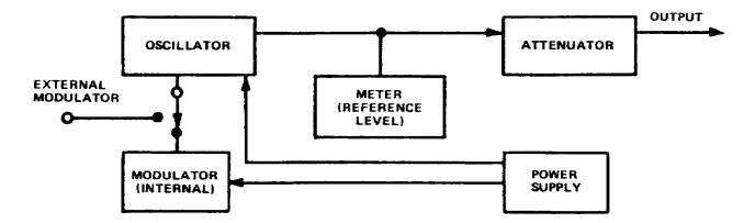
Figure 3-3. Block diagram of RF signal generator
