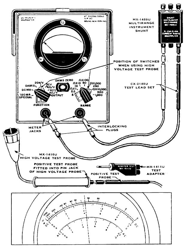
Figure 1-18. ME-70 PSM-6 multimeter
