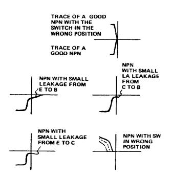
Figure 3-19. Oscilloscope traces of NPN transistors
