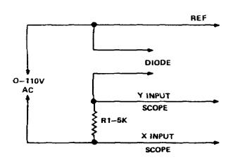
Figure 3-13. Diode tester schematic diagram
