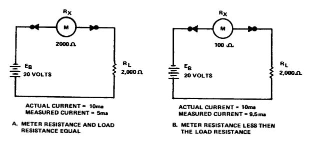
Figure 1-5. Error in ammeter readings
