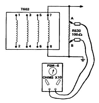
Figure 1-24. Resistance measurement proper circuit conditions
