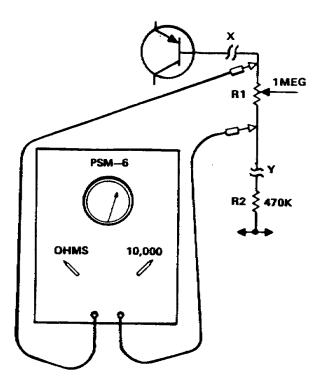
Figure 1-25. Ohmmeter connection
