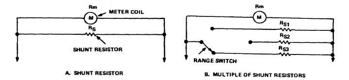
Figure 1-4. Typical ammeter circuit
