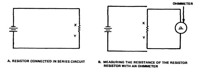
Figure 1-3. Connection of a ohmmeter in a circuit
