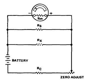
Figure 1-10. A shunt ohmmeter
