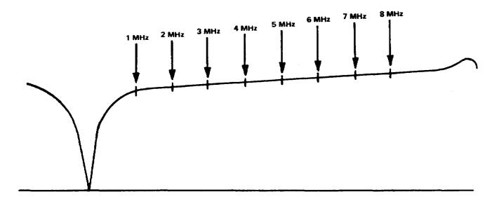
Figure 3-25. Oscilloscope presentation of camera bandpass
