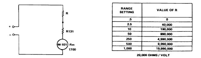
Figure 1-20. 20,000-ohms/volt simplified circuit
