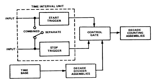
Figure 3-8. Electronic counter time interval measurement, block diagram
