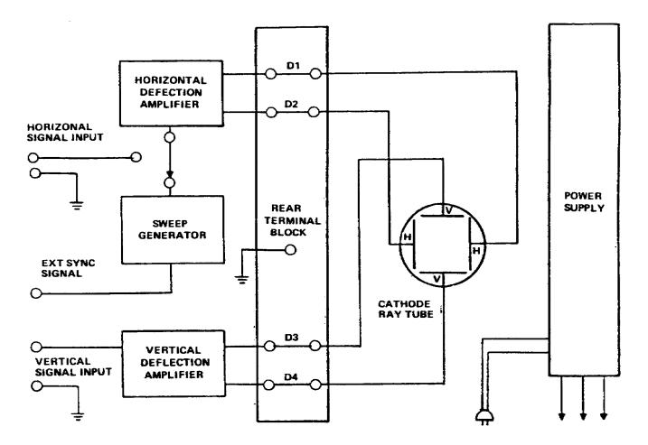
Figure 2-2. Block diagram of a typical cathode-ray oscilloscope
