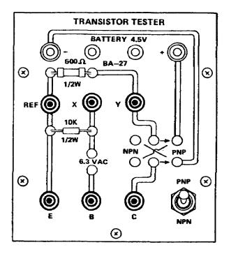
Figure 3-17. Locally manufactured transistor tester
