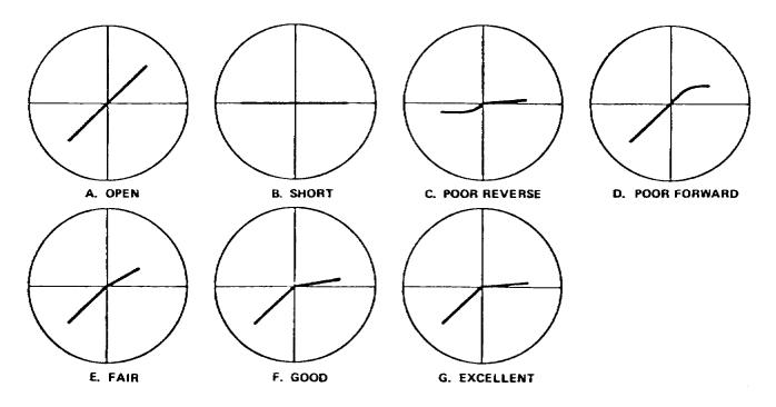
Figure 3-15. Oscilloscope traces of diodes
