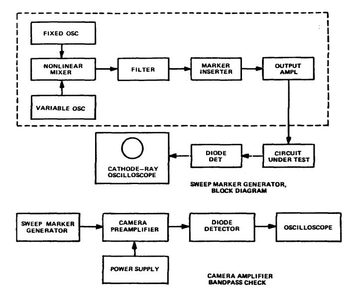
Figure 3-24. Camera amplifier bandpass check
